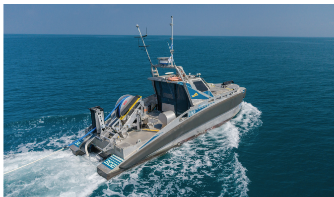
Seagull USV with TRAPS – Towed Reelable Active Passive Sonar
