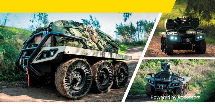
The ROOK is a multipurpose, high mobility 6x6 unmanned ground vehicle (UGV) with all-terrain maneuverability suitable for close and long-range operations under extreme conditions. Designed to carry heavy payloads, the robotic UGV can perform a wide range of urban warfare, battalion maneuvers and border protection missions while increasing front-line effectiveness and survivability.
