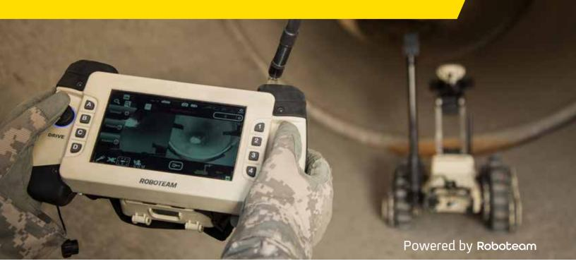
The ROCU-7 (Ruggedized Operator Control Unit – 7" Screen) is a generic, hand-held controller that enables a single operator to control several unmanned systems (land, air or maritime) with one device. Windows based, the ROCU-7 provides complete operational and tactical control, overall mission management and enhanced force coordination. Perfect for military, law enforcement and public safety units, the ROCU-7 helps to create certainty in otherwise unknown spaces.
