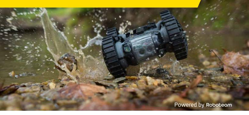
The IRIS (Individual Robotic Intelligence System) is a miniature, rapidly deployable, ruggedized, hand-carried, unmanned system. The system is designed to support units such as SWAT, public safety, military and law enforcement. The IRIS can enter small and confined spaces, above or underground, to explore hazardous areas while relaying intelligence and reconnaissance information in real-time.
