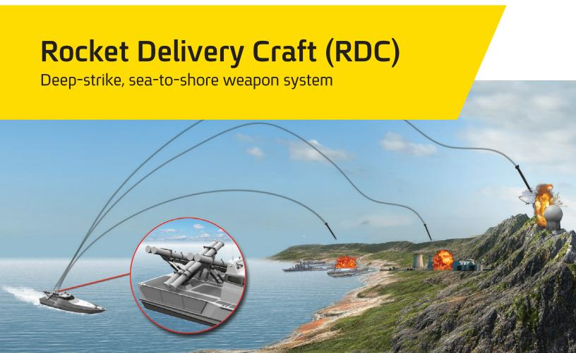
The Rocket Delivery Craft (RDC) is a sea-to-shore weapon system that delivers deep-strike capability against defended targets outside the range of conventional weapons. The 16-meter delivery platform for EXTRA rockets operates from littoral waters beyond enemy weapon range and provides stand-off fight capability. The RDC increases naval independence and enhances naval value in joint multi-branch military operations.
