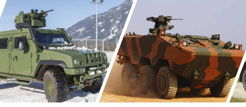
**Dual weapon capability** – The RCWS family includes a dual weapon RCWS with ready-to-fire solutions. The modular design enables multiple weapon combinations, such as 12.7mm MG with 7.62mm MG, 12.7mm with 40mm AGL, or 7.62mm MG with 40mm AGL.
