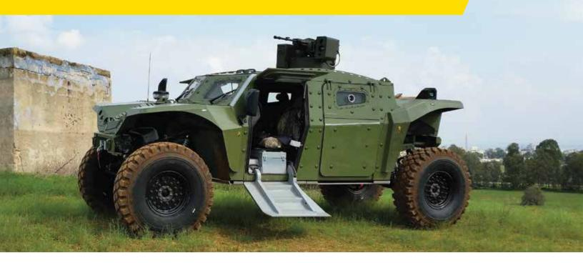
The COMBATGUARD is a high-speed Armored Fighting Vehicle (AFV) with highly protected and extreme off-road capabilities. The unique AFV enables efficient operation in a wide range of combat missions and rough terrains. The high-performance 4x4 AFV can hold a fully equipped crew of six to eight fighters.
