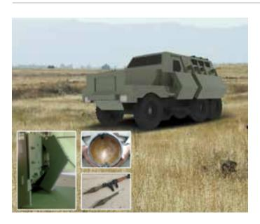
The Breakwater hybrid protection system is based on passive and active armor technologies, designed to minimize the risk of injuring dismounted troops and of collateral damage to non-combatants. The complete armor solution provides a high level of protection against IEDs explosively formed penetrators (EFP) and RPG-7 anti-tank warheads. The shape is optimized to achieve the ideal balance of performance to protect against EFPs and RPGs.
