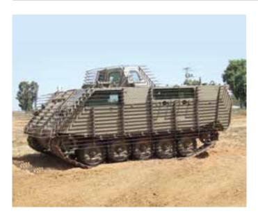
The Urban Fighter suite for M113 provides all-round visibility, advanced firing capabilities and high-level passive armor protection against IEDs, RPG (SLAT), and 14.5mm AP bullets. The vehicle can carry nine fighters with full combat gear.
