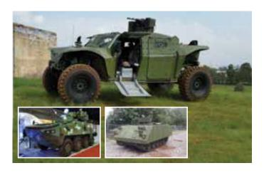
The experience gained with heavy main battle tank (MBT) armor protection has been leveraged and implemented on several lighter platforms. Protection kits developed for the IDF and other customers include systems for the M113 APC and wheeled platforms, such as the CombatGuard, and a tailor-made solution for ICV (8x8 Infantry Carrying Vehicle).
