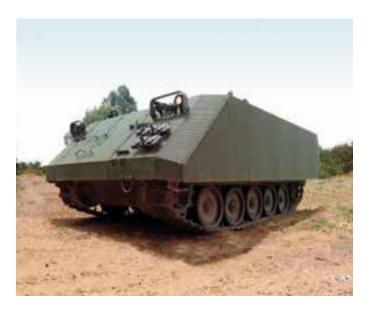
TOGA is an add-on armored solution composed of specially perforated steel plates. The cost-effective solution offers low-weight protection for APCs against AP bullets, and artillery and shell fragments. The add-on armor provides high-level ballistic protection (350% efficiency) by deflecting the bullets' trajectory and protects against RPGs by reducing the dispersion. TOGA is type-qualified and fielded by the IDF and other forces worldwide.
