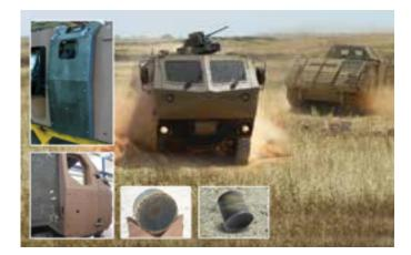
Iron Wall is a combat-proven innovative passive ballistic structure capable of defeating medium IED threats, such as explosive flyer plates EFPs and steel-ball charge focus fragments SFFs. The solution provides passive add-on armor comprising a combination of composites and metals. The protection system is compatible with medium and light platforms (tracked or wheeled APCs).
