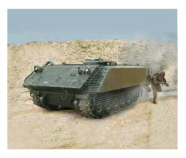
The light vehicle armor system (LVAS) is based on modules that are easily replaceable in the field, providing low weight protection against multiple threats: RPG-7 warheads (perpendicular hits), IED and artillery fragments, 7.62mm and 14.5mm AP bullets. With optimal explosive and metallic contents, the add-on hybrid (passive and reactive) modular armor system is a reliable and safe solution for APCs crew and deployed troops.
