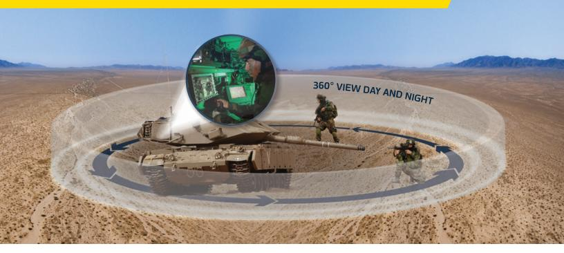
Elbit Systems' See-Through Armor (STA) creates a new level of situational awareness and operational efficency under closed hatches. Utilizing a set of high-resolution day and night cameras, the STA provides a full view of the battlefield, without compromising crew safety.
