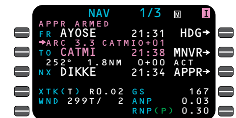
The RNP associated with the current leg is displayed on the NAV pages. The RNP value is obtained from the navigation database when provided for that leg; otherwise it is the FMS default value for the current phase of flight.
