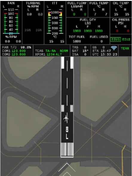
MFD with Taxi View and Engine Display
