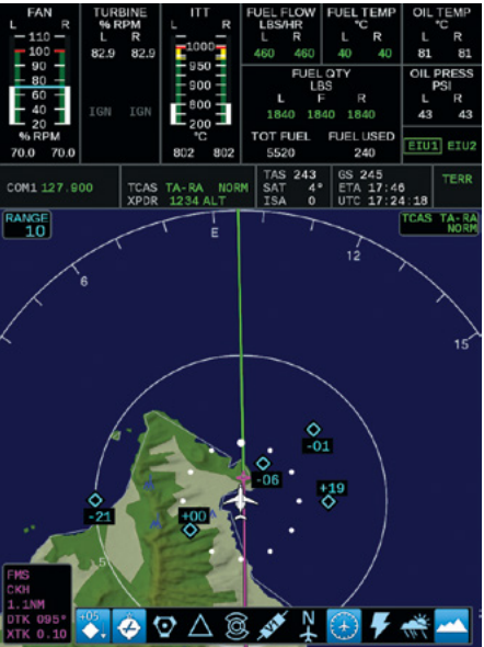
MFD Full Format with Compressed Engine Display
