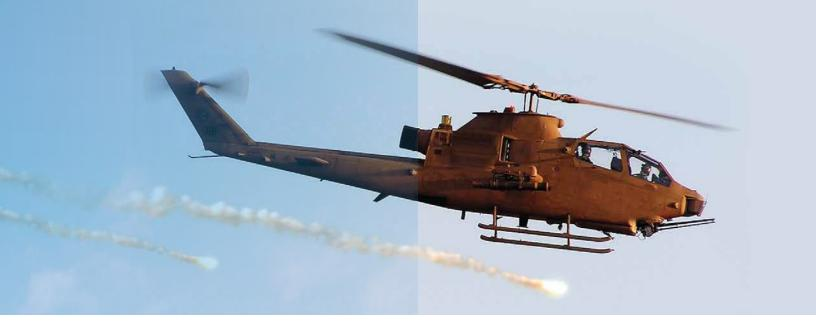
**System integration and compatibility:** The MINI-SAMP is available as a complete system installed on aircraft or as an upgrade kit for retrofitting existing Countermeasure Dispenser Systems (CDMS) already in use. The system is fully compatible with all aircraft systems (discrete lines, RS-422 serial communication, MIL-STD-1553 multiplex data bus). The cockpit control unit is compatible with Night Vision Goggles (NVG).
